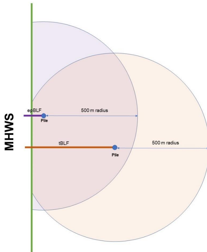
Figure 6.1 Schematic illustration of the mitigation zones for the enhanced permanent BLF and temporary BLF MBIF in relation to the MHWS (please note, the pile positions were located at the furthest point from MHWS i.e., radius has been applied from the terminus of the BLFs BLF and MBIF).
